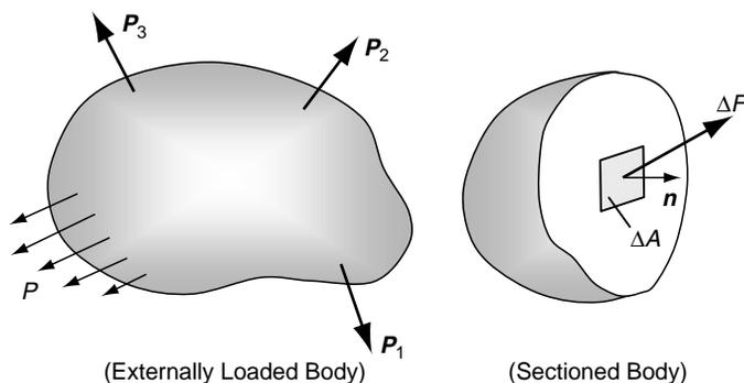
FIGURE 3-2 Sectioned solid under external loading.
