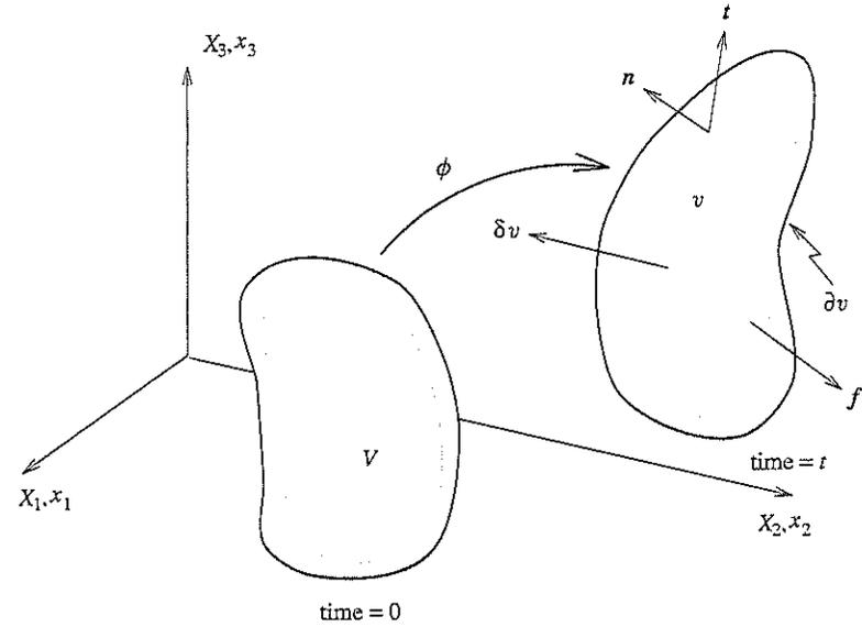
FIGURE 4.6 Principle of virtual work.
