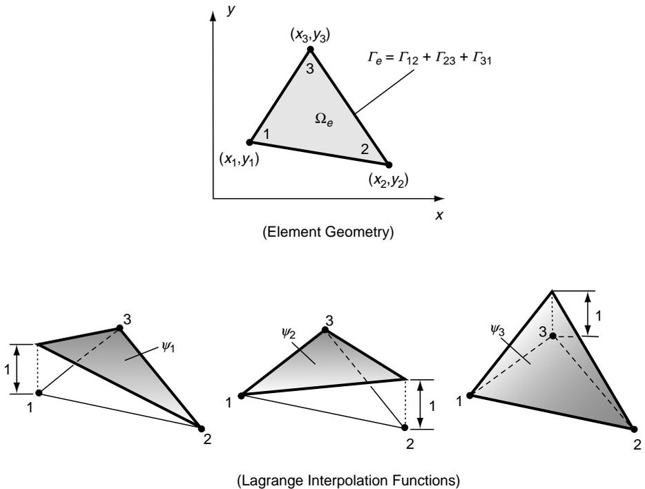
FIGURE 15-2 Linear triangular element geometry and interpolation.
