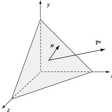
FIGURE 3-4 Traction on an oblique plane.
