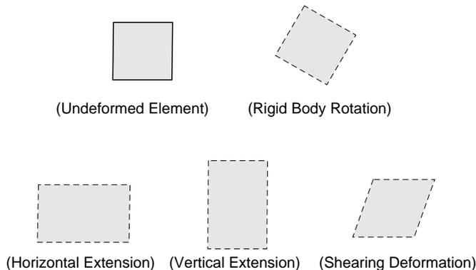
FIGURE 2-3 Typical deformations of a rectangular element.
