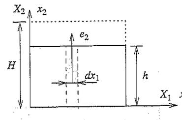
A simple example of a two-dimensional stress tensor results from the self-weight of a block of uniform initial density  $\rho_0$  resting on a frictionless surface as shown in the figure above. For simplicity we will assume that there is no lateral deformation (in linear elasticity this would imply that the Poisson ratio  $\nu=0$ ).
