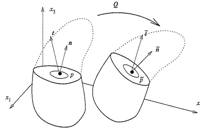
FIGURE 4.4 Superimposed rigid body motion.
