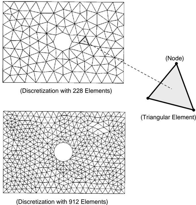
**FIGURE 15-1** *Finite element discretization using triangular elements.*
