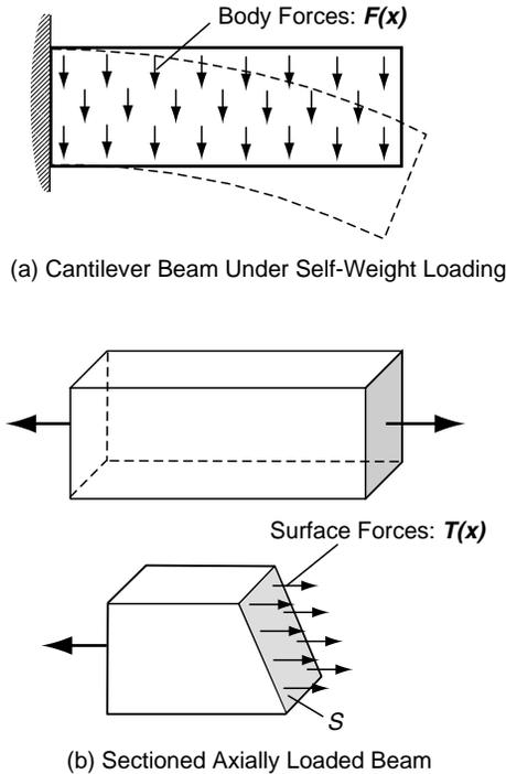
FIGURE 3-1 Examples of body and surface forces.
