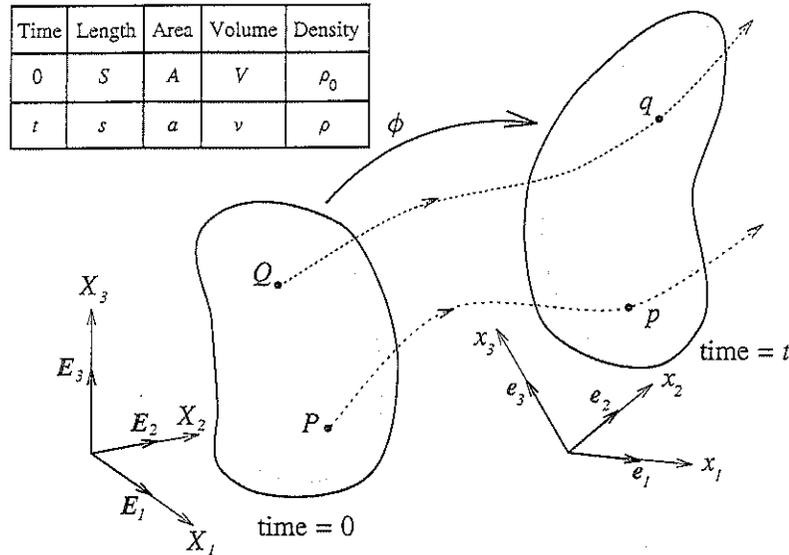
FIGURE 3.1 General motion of a deformable body.
